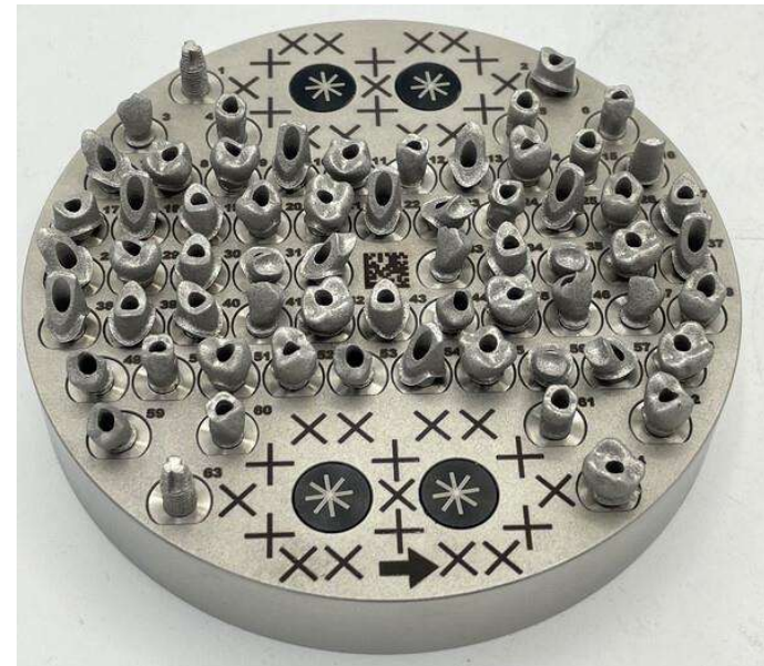
Custom and serial 3D print abutments (Titanium Grade 23) Made by the TRUMPF Preform Technology
